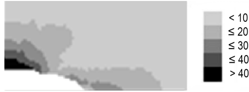
Figure 1: Distribution of stress intensity near an elliptical hole ( r_2/r_1 = 1/8 ).
